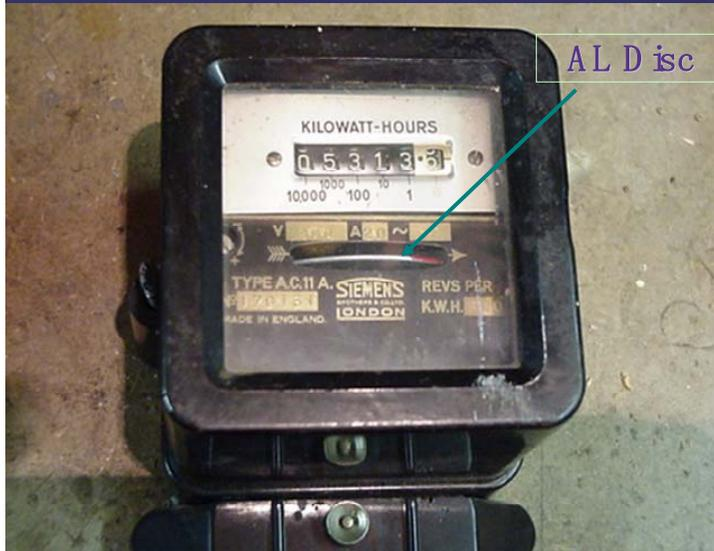
Voltage and Current pass through electromagnets, generating FLUX, which develops Torque which in turn Rotates AL Disc.
